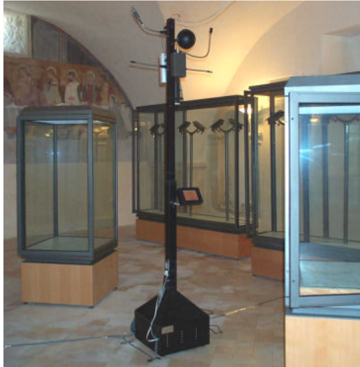
Fig. 4. Prototype of innovative integrated monitoring system during the museum room preparation phase (realised by ITC-CNR)
