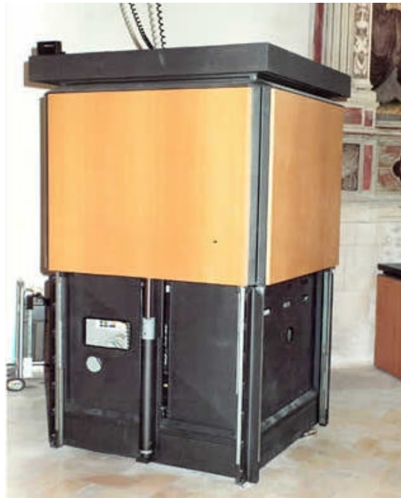
Fig. 3. Innovative system for exposed works of art protection from the effects caused by earthquakes during normal working conditions and after a warning situation (realised by Borini Costruzioni)
