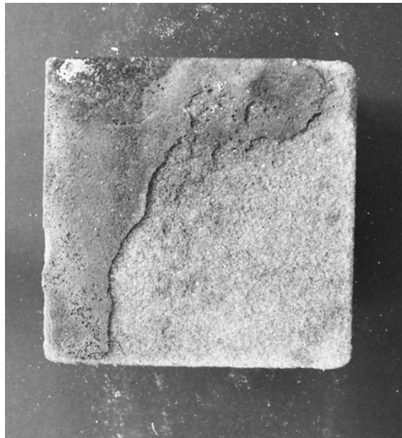
Figure 4 A block of sandstone subjected to real fire and salt weathering simulations in the laboratory. The less permeable soot crust has detached as a result of salts concentrating and crystallizing behind it, exposing more permeable, fire-damaged, sandstone beneath. The exposed stone exhibits rapid granular disaggregation as a result of exploitation by salt weathering.
