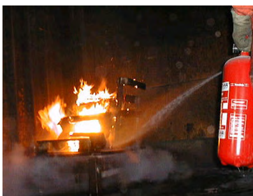
Figure 4: Water extinguisher in test
