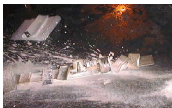
Figure 7: Test set with 13 different museum objects is sprayed with aqueous film forming foam following exposure to smoke from a Class A fire at about 200 °C
