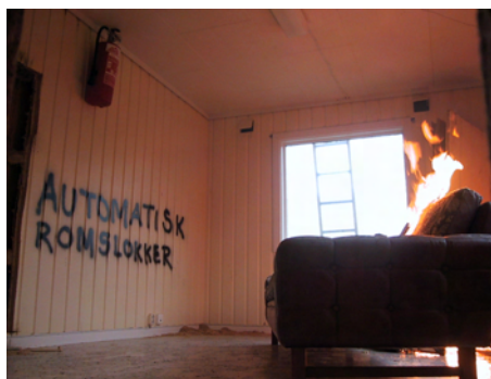
Figure 12: Realistic performance test of ceiling category automatic extinguisher (COWI AS)
