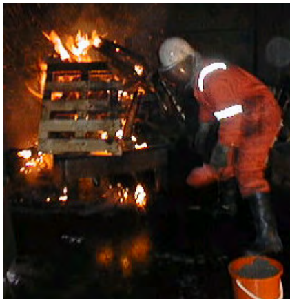
Figure 11: Sand applied in extinguishing performance test. The sand used was too wet for successful application.
