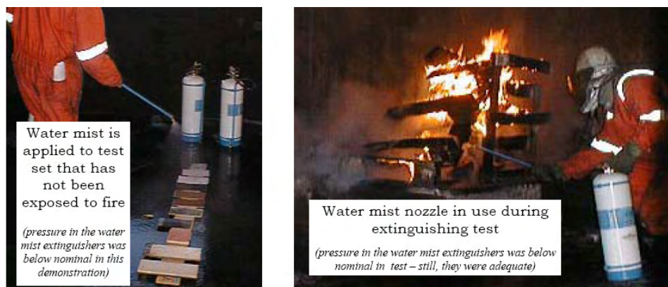
Figure 5: Water mist extinguishers applied to material samples not exposed to fire, and in extinguishing test.
