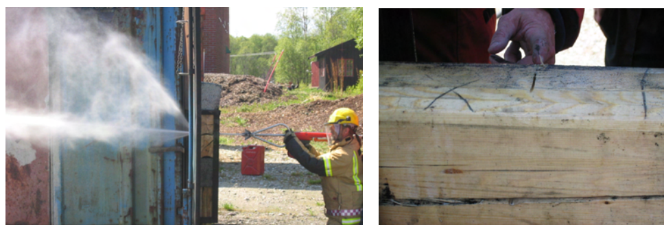
Figure 13: Piercing high pressure water mist nozzle during performance demonstration. Log wall is penetrated. Note 2 mm diameter tracks by penetrations at joints.
